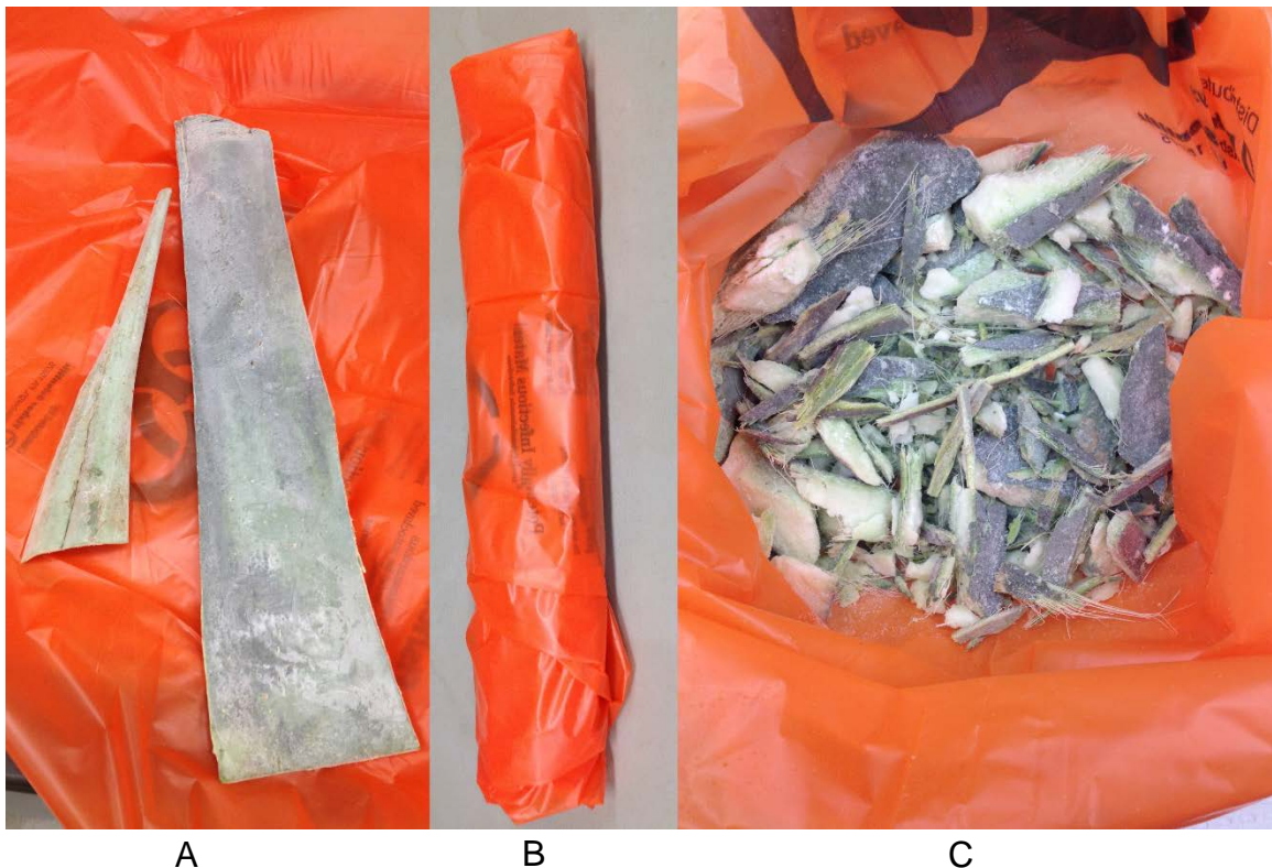
Figure 4. Breaking up of Agave tequilana leaves. (A) Two large frozen pieces of Agave tequilana leaves, (B) large leaf pieces wrapped in 3 biohazard bags, (C) frozen broken up Agave tequilana pieces ready to be weighed and added to fermenters.
