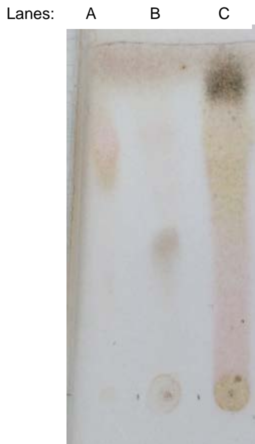
Figure 23. TLC of mycosporine-like-amino acid extracts from seaweed (lanes A and B) and Agave tequilana skin (lane C) after sulfuric methanol detection spray for hydrocarbons.
